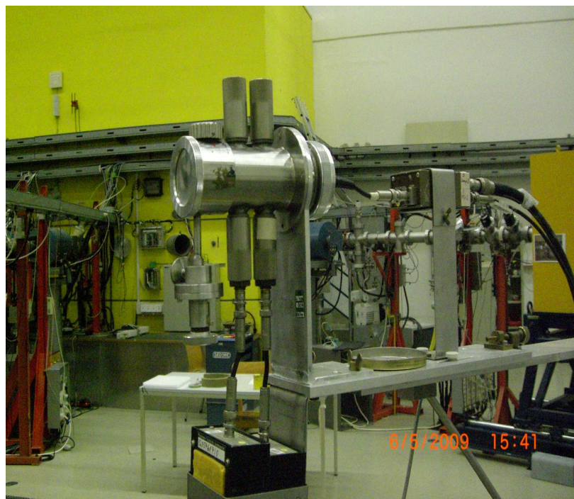
Proton recoil telescope (fluence measurement relative to n-p scattering)
